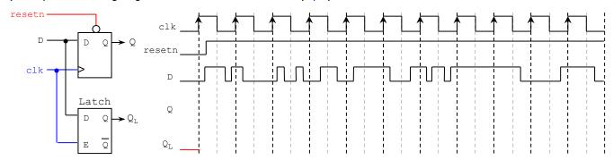
b) Complete the timing diagram of the circuit shown below: (6 pts)
